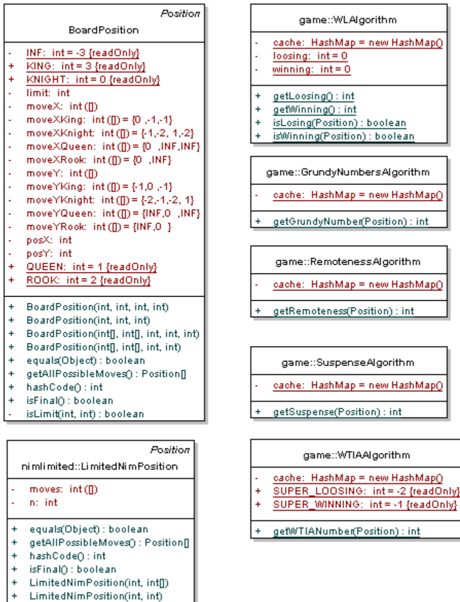
Figure 14: UML class diagram for the games NimLimited and Board Games on the left and class diagrams of algorithms in package sk.lenhardt.game on the right
